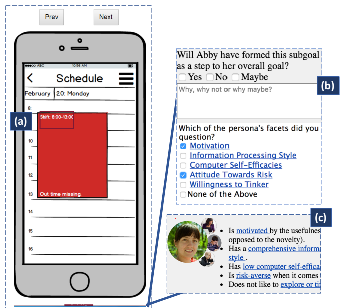
Fig. 3: The Recorder’s Assistant tool during an evaluation of a mobile time-and-scheduling app. (Left): The app being evaluated is displayed with (a) a rectangle around the action the evaluators are deciding if a user like “Abby” will take. (Right): A blow-up of portions of the GenderMag features for the app: (b) the GenderMag question the team is answering at the moment, including a checklist of Abby’s facets; and (c) a summary of the persona the team has decided to use (in this case, Abby).
