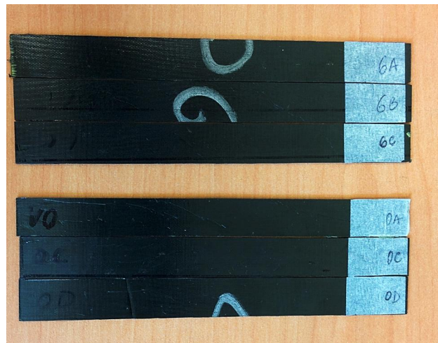
Figure 4.6: Final impact test specimen
