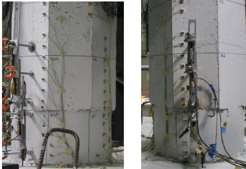
Figure 3.7 Optotrak sensor configuration on the test specimen. On left is a view of north and west sensors. On right is a view of south sensors.
