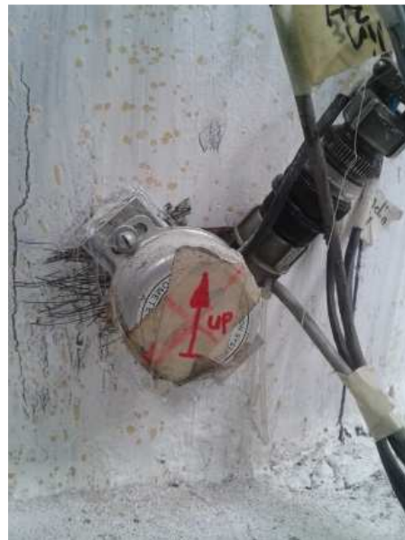
Figure 3.8 Typical inclinometer attached to the column's east face.
