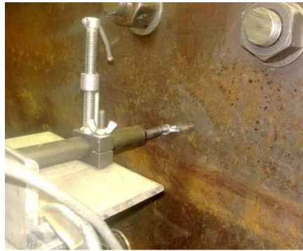
Figure 3.10 The LVDT used to measure the actuator beam deflection during testing.
