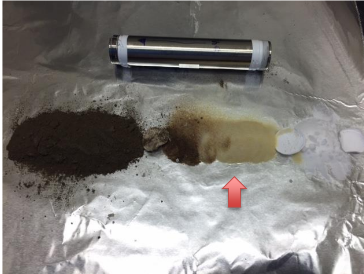
Figure 9. Emptied contents of an extracted ASE cell. Starting from the top (left) is the sediment, GF/F filter, sulfuric acid activated silica gel, GF/F filter, neutral silica gel, and a last GF/F filter. The yellow portion of the sulfuric acid activated silica gel was not seen before samples started containing hydrocarbon oil.
