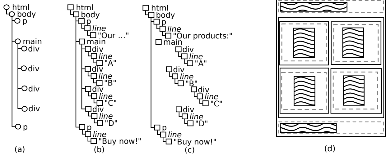
Figure 2.1: Layout converts HTML into a tree of elements (2.1a). The tree of elements generates a tree of boxes (2.1b), which includes block, line, and text boxes, and this tree is broken into flow trees (2.1c). A position and size is then computed for every box, resulting in the layout (2.1d).
