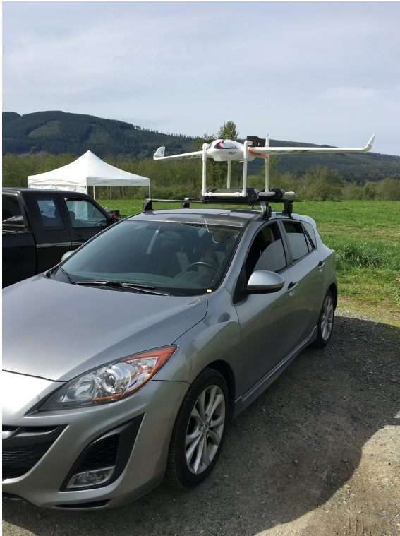
Figure 3.8: HAPRA mounted for a driving test on April 16th at Meadowbrook Farm
