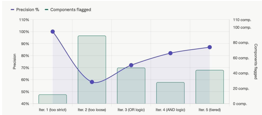
Figure 3.1: Threshold calibration progression showing precision improvement and components flagged across five iterations
