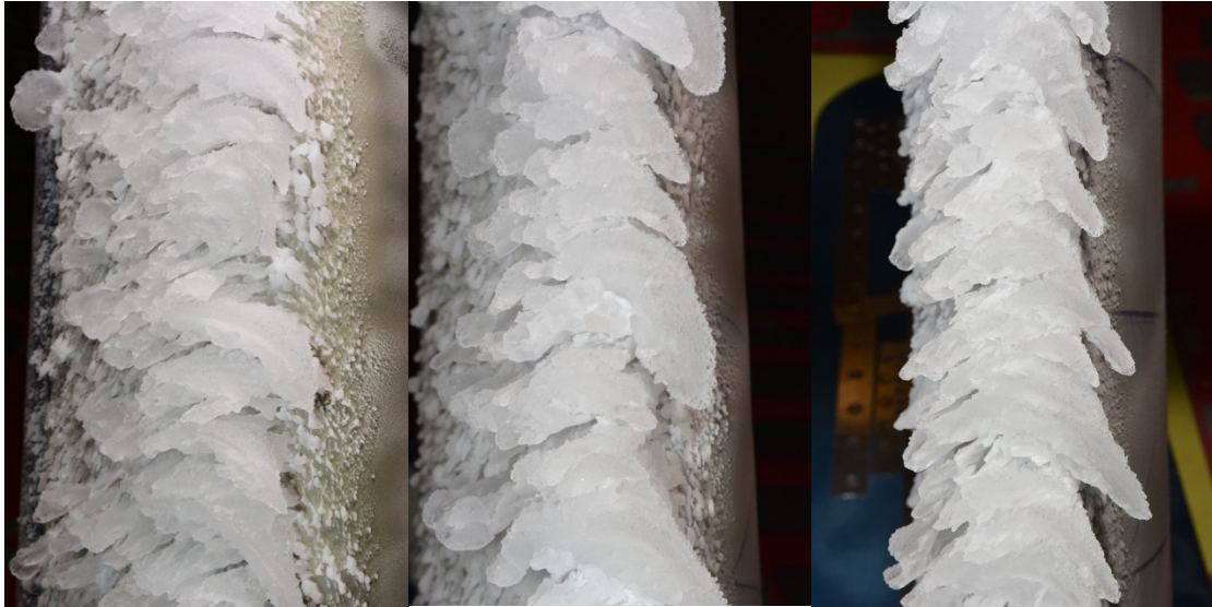
a) Inboard, Midspan, and Outboard model ice accretions, respectively courtesy of Camello et al. [25]
