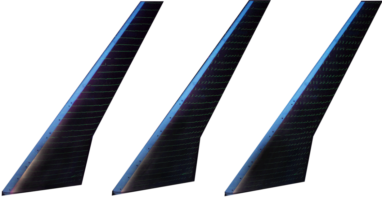
Fig. 3.19 Maximum Scallop fluorescent mini-tuft visualization at Re = 1.6 \times 10^6 and M = 0.18 for \alpha = 4.8^\circ , 7.9^\circ , and 8.9^\circ , respectively.
