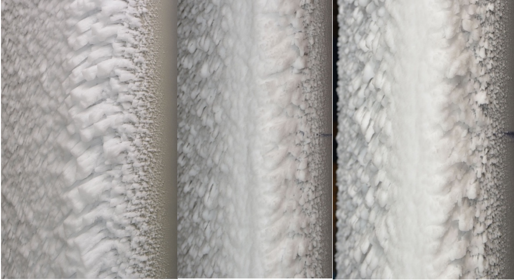
a) Inboard, Midspan, and Outboard model ice accretions, respectively courtesy of Camello et al. [25]
