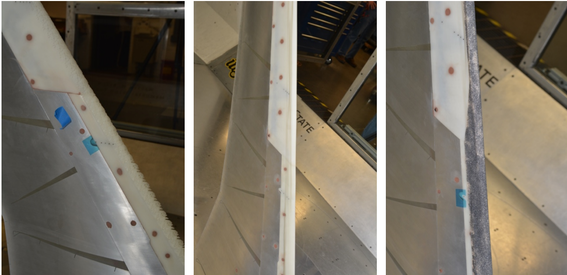
Fig. 3.21 Shown left to right; High fidelity, 2D smooth, and 2D smooth + grit Maximum Scallop artificial ice shapes installed on the 8.9% scale CRM65 wing.
