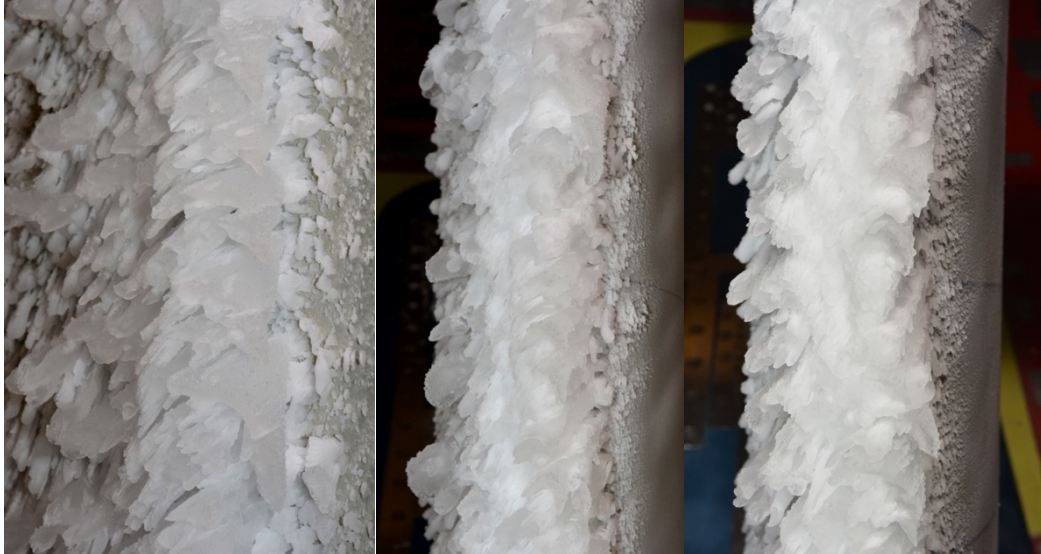
a) Inboard, Midspan, and Outboard model ice accretions, respectively courtesy of Camello et al. [25]
