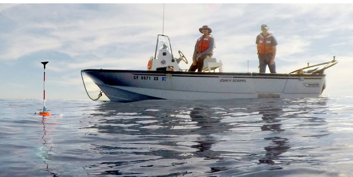
FIGURE 1. F\chi S is flipped, ready to communicate with the antenna pointed up, and ready to descend with the sensors pointed down into the clean flow during a test off San Diego.
