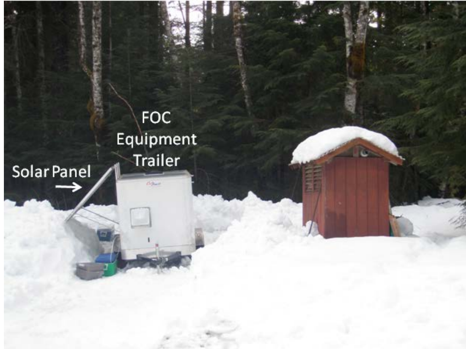
Figure 3.11 Photograph of the equipment trailer and solar panel used to power and operate the FOC. View is toward the southwest, with the Bear Creek intensive gap plot in the forest shown in the background. Partway through the deployment, the trailer was moved further away from the trees in an attempt to reduce the time during which the solar panel was shaded each day.
