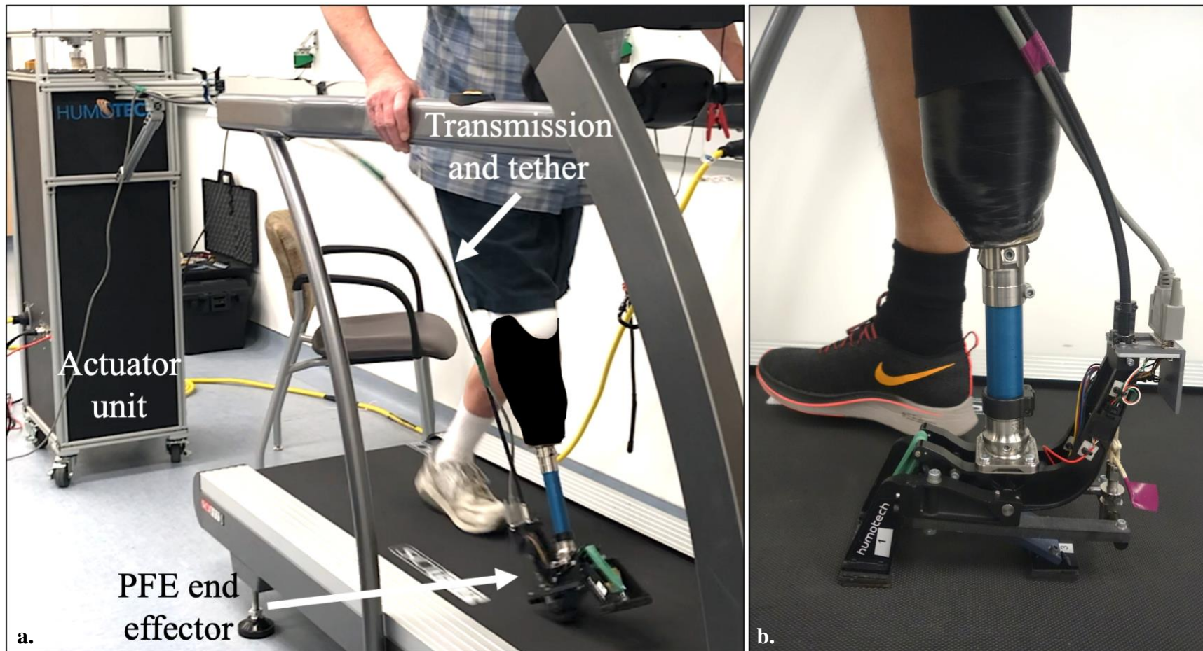
Figure 2.1. a) Photo illustrating a user with transtibial amputation with the PFE end effector attached to their socket and tethered, offboard actuator unit and control hardware depicted behind the user; b) photo of PFE end effector attached to socket of participant with transtibial amputation.
