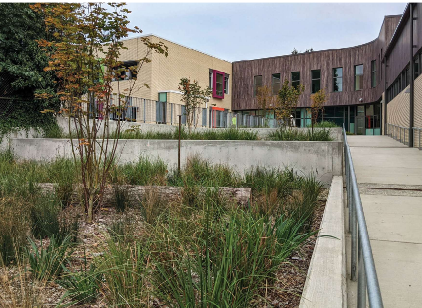
Fig. 5.20: Bioretention area (Fora Landscape Architects)
