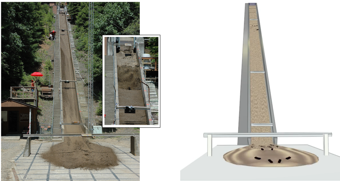
Fig. 9.12. Digital twin of the USGS Volcanic Hazard Program's lahar flume during a dry sand-gravel experiment. Digital twin implemented in ClaymoreUW for the Material Point Method.
