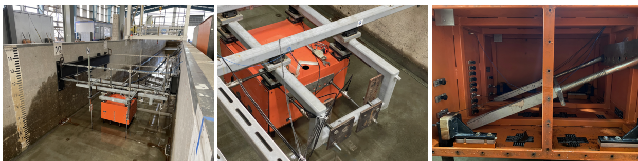
Fig. 7.5. Raised structural box used in OSU LWF debris-field tests. The raised "orange box" from Winter 2019 , Shekhar et al. 2020 , and Mascarenas 2022 which is used to measure wave and debris loads. Interior stiffened with cross-bars.
