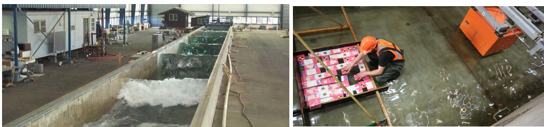
Fig. 7.3. Photographs of Oregon State University's large wave flume. (Right) OSU LWF with large breaking waves. (Left) Preparing random debris test in front of the orange structural box.
