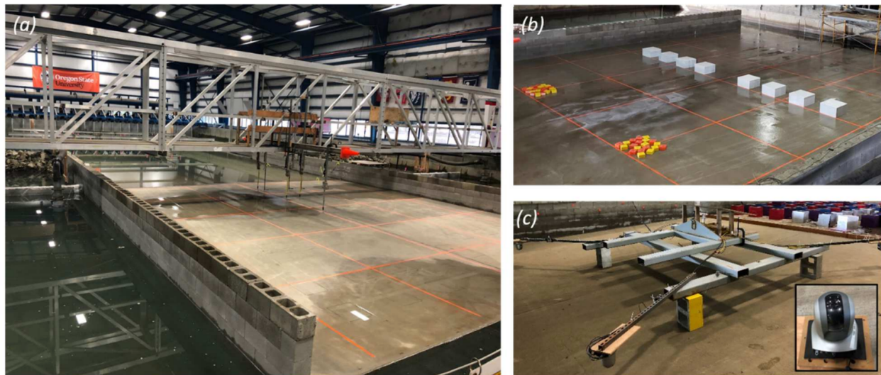
Figure 2: Photographs of the debris test setup. (a) Overview of testbed without debris, (b) Overview of the testbed in other direction with two setups of debris and eight obstacles, (c) Steel frame for the camera mounting and snapshot of the camera (inner photo).
