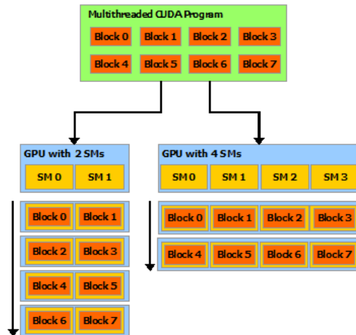
Fig. 3.3. Scaling across streaming multiprocessors. Blocks automatically distribute across streaming multiprocessors. Courtesy of NVIDIA.
