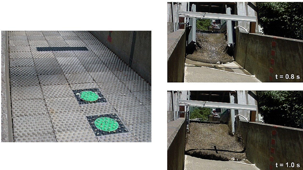
Fig. 9.14. Photographs of Iverson 2010 debris-flow experiments. Soil mass consisting of sand, gravel, and mud as it is released by swinging gates at the top of 31 degree sloped flume. Portions of flume have "bump pads" (grey) to replicate prototype slope roughness. Load-cell ports have sides of 34cm (black), load-cell faces are 25.2 cm (green).
