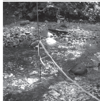
Conservative tracer injection setup. The NaCl mixture (top) is pumped through a tube (middle) to a mixing zone in the middle of the stream (bottom).
