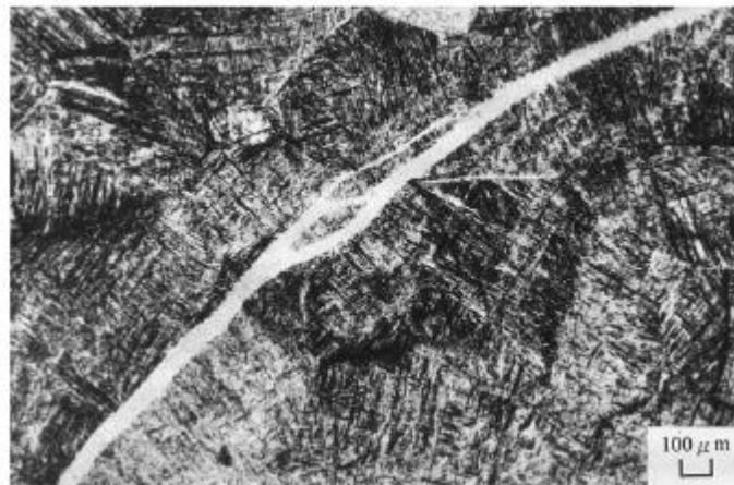
Figure 1-12: Adiabatic shear band obtained at strain rate of 2 \times 10^3 \text{ s}^{-1} at 1100^{\circ}\text{C} [Lee, 1998].
