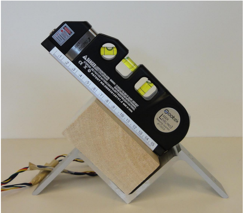
Fig. 4.2. “Box” experiment in a 45° orientation, supported by steel angles
