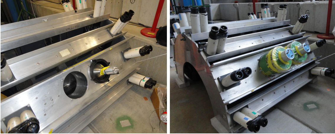
Figure 4.5: Bicorn (left) and DEMON (right) neutron detectors mounted to eSC frame.
