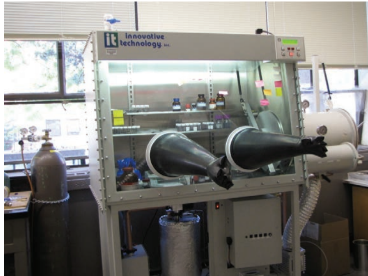
Figure 1.11: box system at Ar atmosphere
