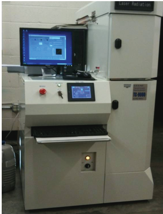
Figure 1.12: Laser flash measurement system: Thermal diffusivity and specific heat capacity are measured simultaneously (TC-9000, Ulvac-Rico)
