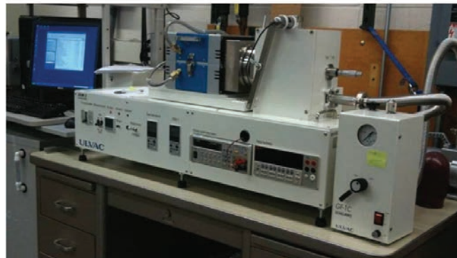
Figure 1.13: Four-point probe system: the measurement of Seebeck coefficient and electrical conductivity (ZEM-3, Ulvac-Rico)
