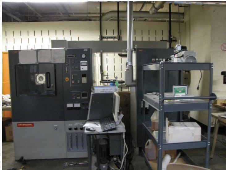
Figure 1.10: Spark plasma sintering equipment (Dr. Sinter 1020S, Sumitomo Coal Mining Co., Ltd.)
