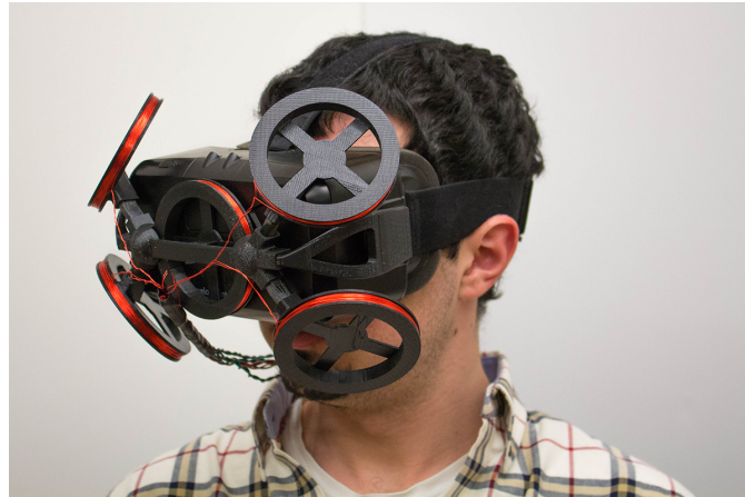
Figure 3.1: The EyeContact scleral coil tracker can clip to an HMD and does not require the use of a head mount or room-sized field coils
