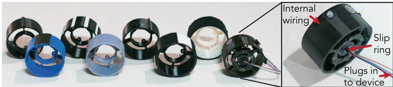
Figure 6.5: Interchangeable haptic wheels allow applications to customize the haptic experience with various shapes and textures. (right) Wheels with active components use a slip ring in the wheel mount to wire the electronics in the wheel back to the device.
