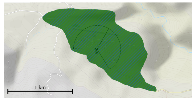
(d) Interpolated coverage map from walk testing. The hashed green area indicates measured satisfactory coverage ( -110\text{dBm} RSRP "two bars" or greater), capable of saturating the satellite backhaul link. Map data from OpenStreetMap [132]
