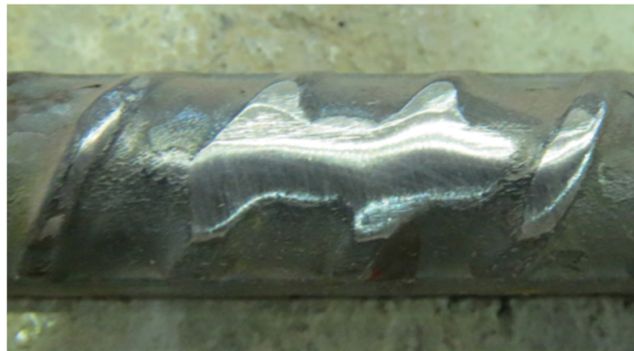
Figure E.1 Milled and polished spot on rebar for application of strain gauge.
