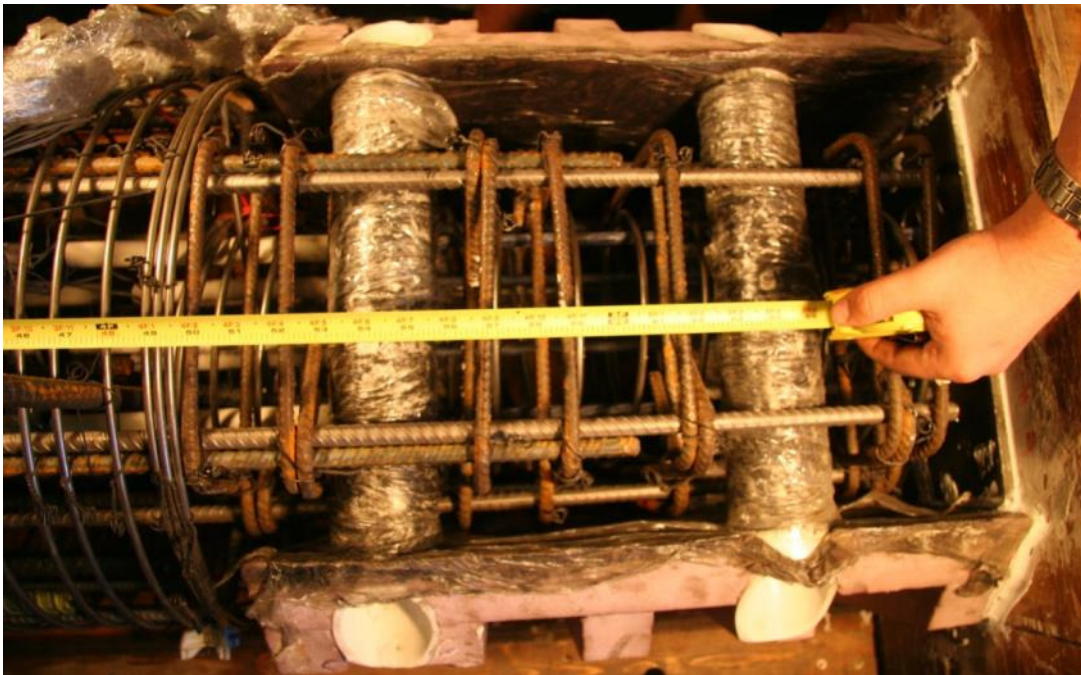
Figure D.3 Reduced depth segment for actuator attachment.
