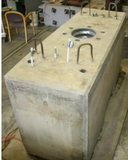
Figure D.11 Cast cap beam isometric view.
