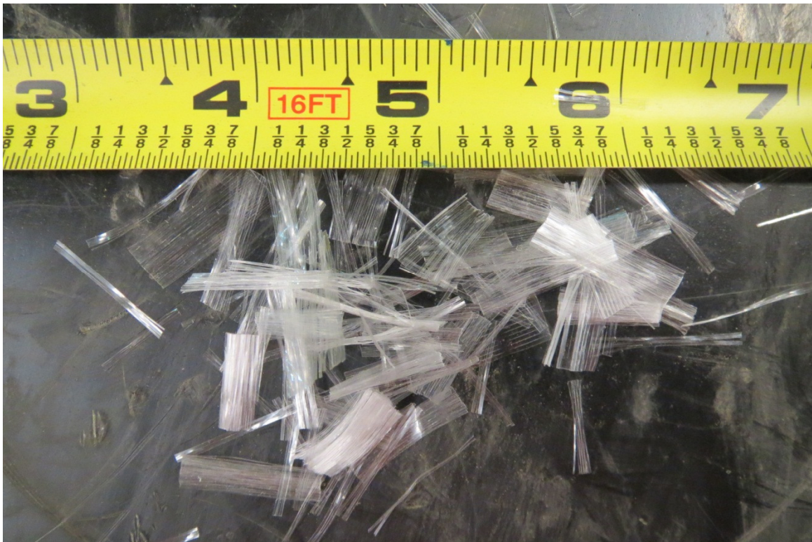
Figure 2.18 Fibermesh 300 polypropylene fibers used for grout pad.
