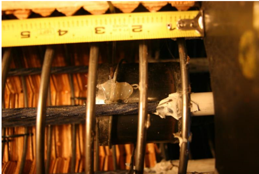
Figure D.5 Tubular housing for dowel bar.
