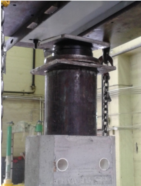
Figure 3.3 Bearing assembly with stand-off on top of PreT-SF-ROCK (Schaefer et al., 2014a), an identical setup was used for the PreT-CB-COCK test.
