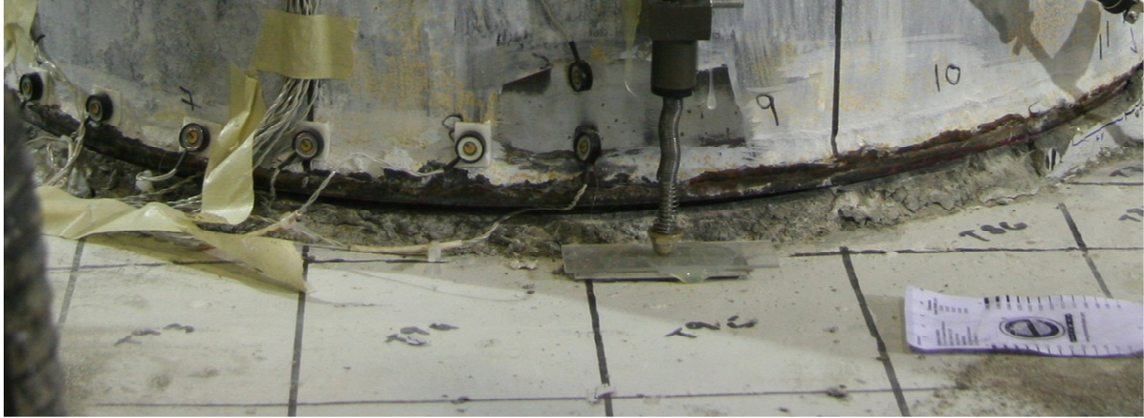
Figure 4.12 Minimal grout crushing after \pm 10.41\% drift cycle (Set 10-Cycle 3) -- before initiating the cycle, the previously crushed grout was removed.
