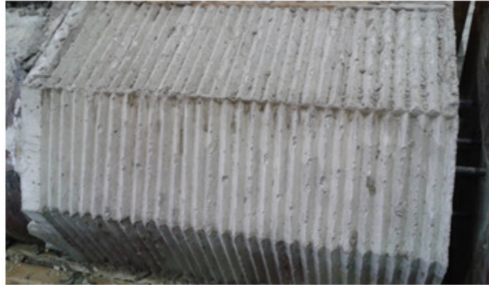
Figure 6.39 Bottom, 20 in. wide octagonal section of PreT-SF-ROCK (Schaefer et al., 2014a).
