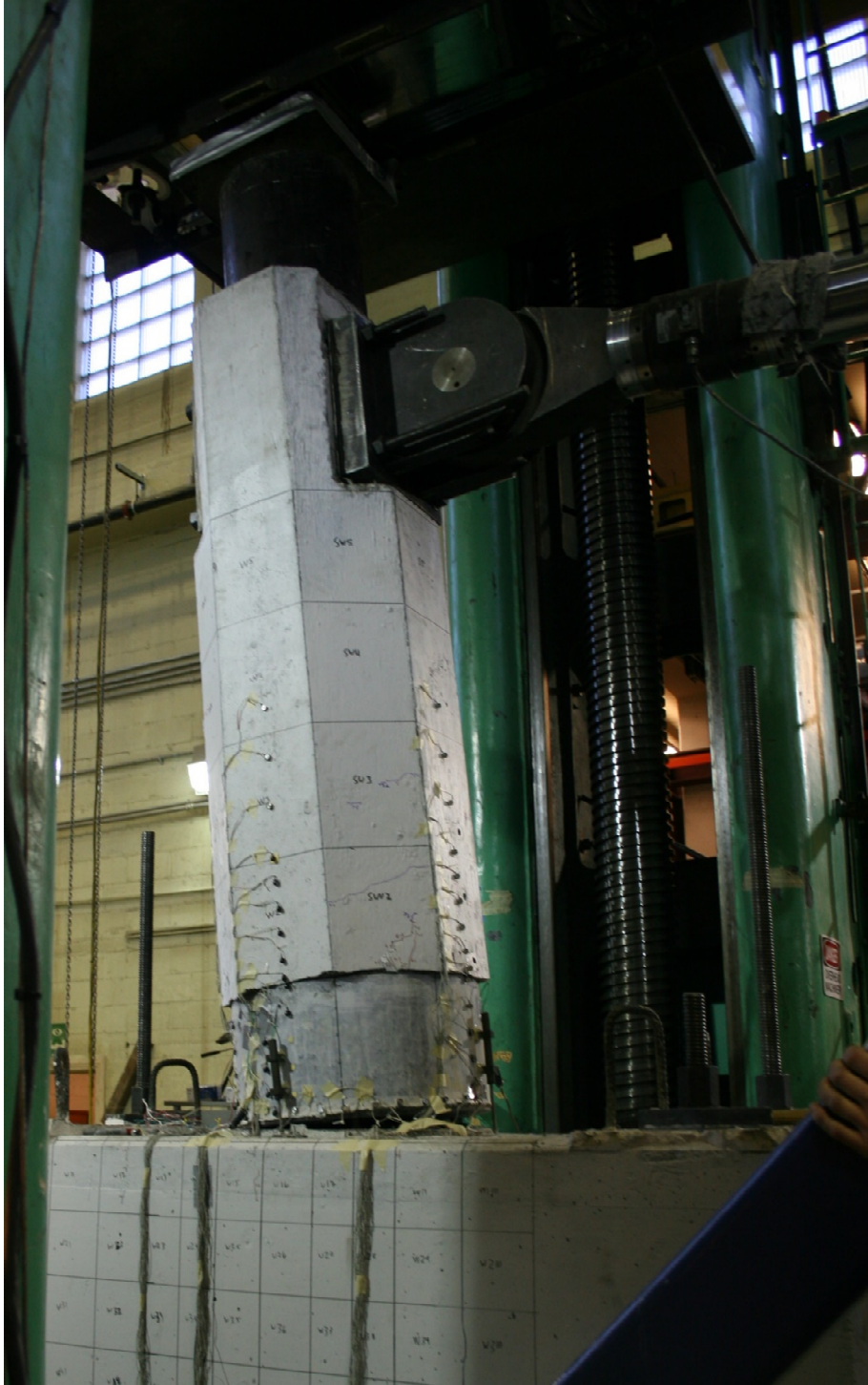
Figure 4.2 PreT-CB-ROCK being displaced to the minimum valley drift of the test (photo taken from southwest of specimen).
