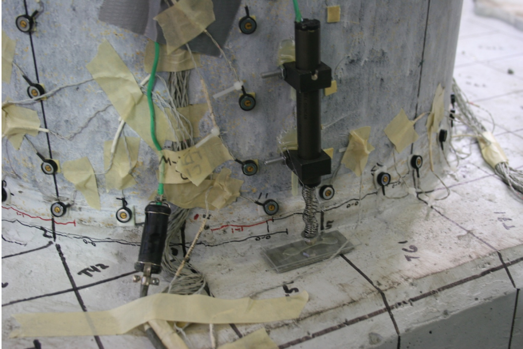
Figure 3.5 Linear potentiometer used to measure movement of steel tube.
