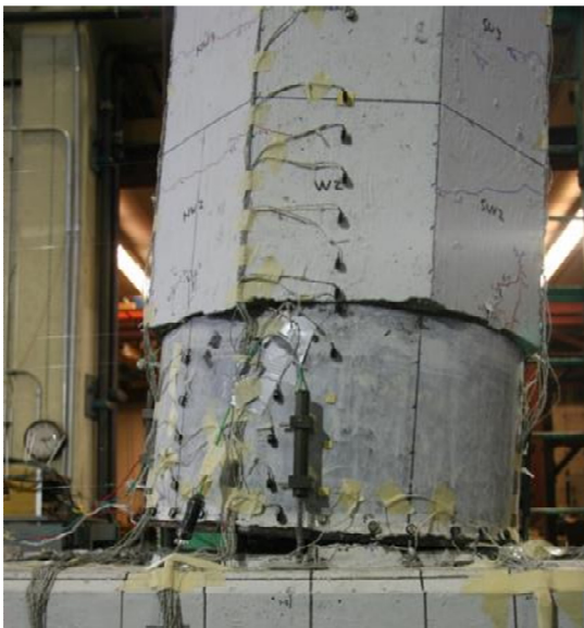
Figure C.2 Column rocking during peak (left) and valley (right) displacements of maximum drift ratios of test ( \pm 10.41\% ).
