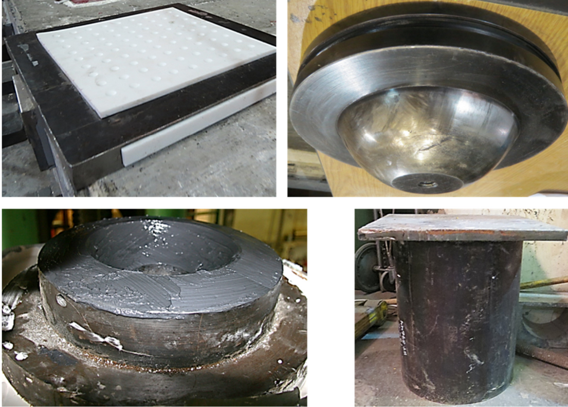
Figure 3.2 From upper-left: PTFE clad bearing plate, ungreased top spherical bearing, greased bottom spherical bearing, and standoff used to transfer the vertical load from the Baldwin.
