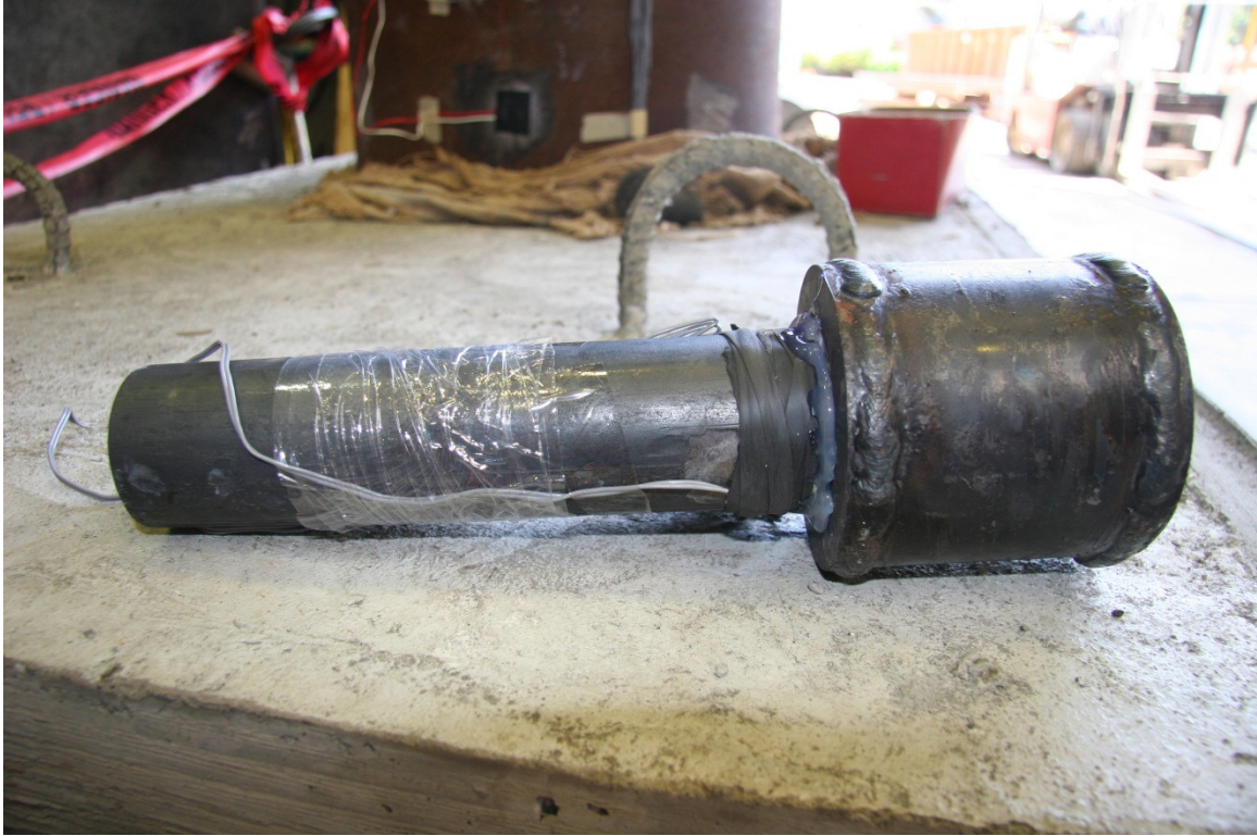
Figure 2.11 Dowel bar and housing fixture.
