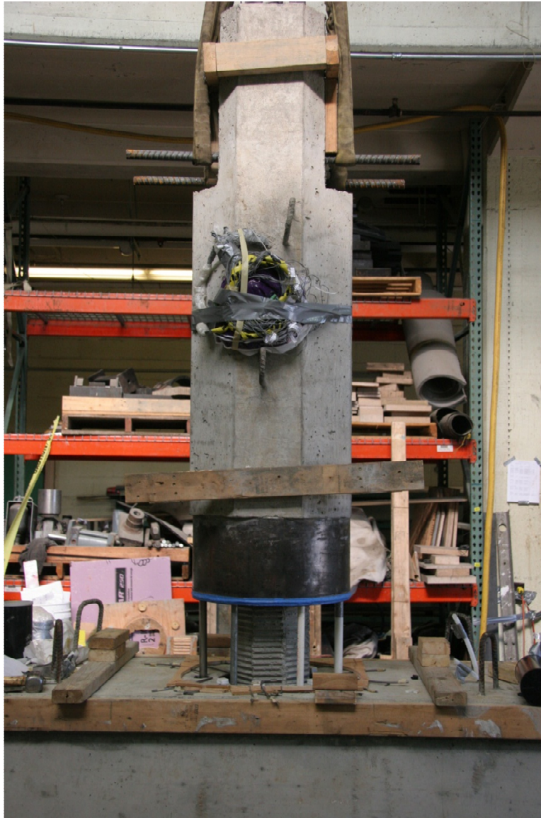
Figure 2.23 Fitting of the column-to-cap beam socket connection.
