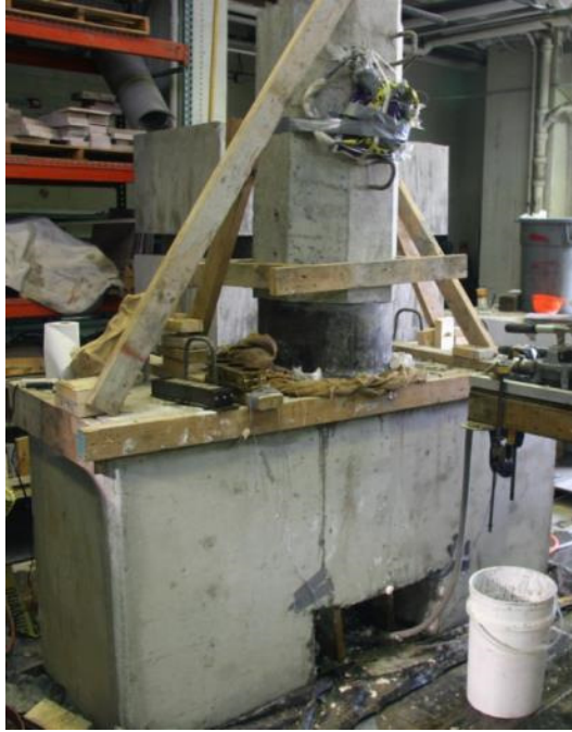
Figure D.17 Specimen during grout pumping operation.
