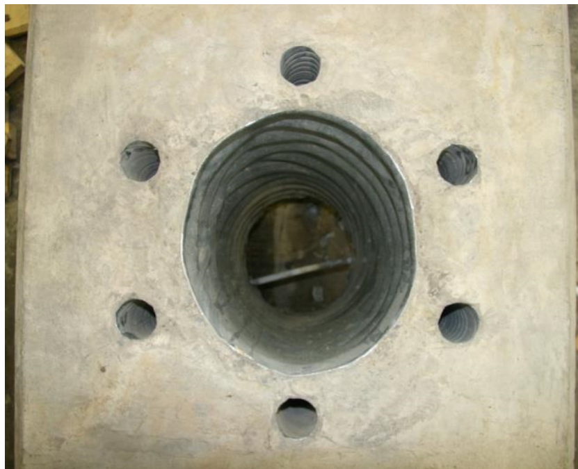
Figure D.12 Socket connection ductwork.
