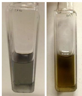
Figure D.6. Coloration of ZnO nanocrystal suspensions when exposed to UV illumination in the presence of Li[Et 3 BH] or Li[Me 2 NBH 3 ].
