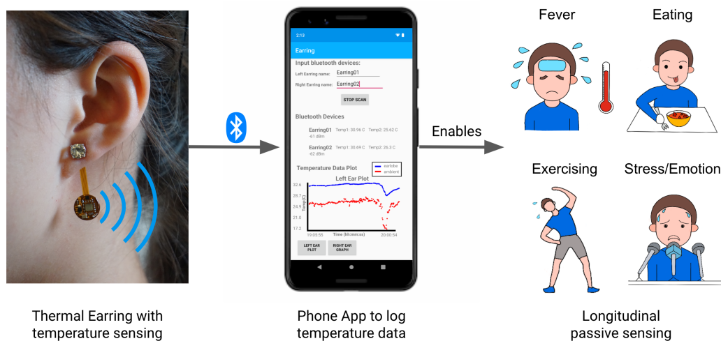
Figure 3.1: Thermal Earring is a first-of-its-kind smart wireless earring that enables a reliable wearable solution for continuous temperature monitoring. By leveraging the earring’s unique position near the head, it significantly improves temperature sensing accuracy, enabling new health applications such as continuous fever monitoring, eating and exercise detection, acute stress detection, and women’s cycle tracking.
