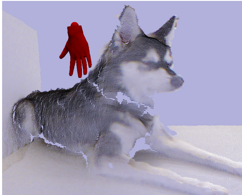
Figure 6.1: An application to six degree-of-freedom haptic rendering from streaming point clouds: Petting a point cloud representation of a dog captured using the Kinect. The virtual tool representing the haptic device in the virtual environment has the form of a human hand.
