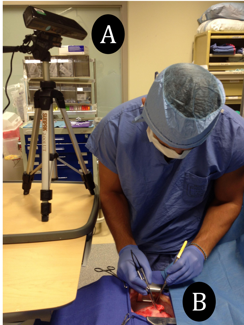
Figure 5.7: Capturing the RGB-D data. The Kinect camera (A) was located directly above and looking down at the heart (B). This position and orientation was chosen since it resulted in a very good depth estimation (a dense point cloud). The haptic device is not shown in this figure.
