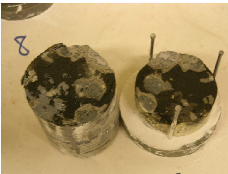
Figure 6-1. Typical Editaan Tensile Failure. The dark area is Editaan and the lighter patches are lightweight concrete.
