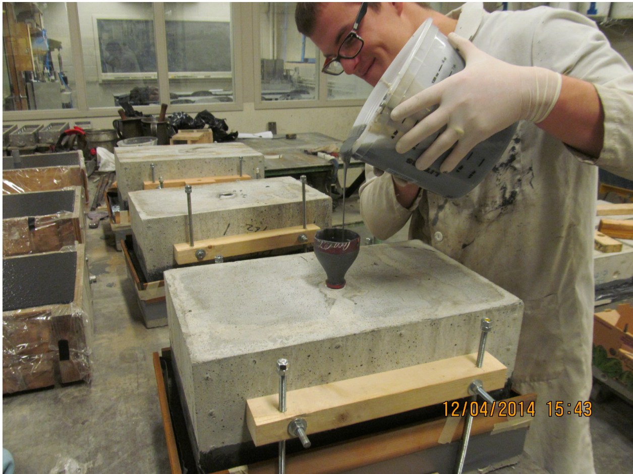
Figure 4-7. For the full-size plinths used in compression testing, the DexG was poured through a central blockout, flowing radially outward under the block.
