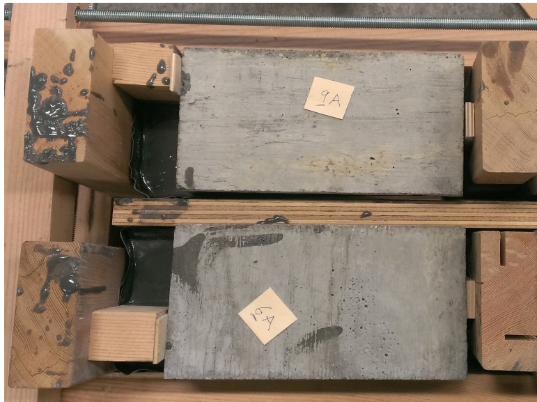
Figure 4-4. Two shear specimen during DexG Application. The DexG flows from the large dam on the left underneath the lightweight concrete block to the right.
