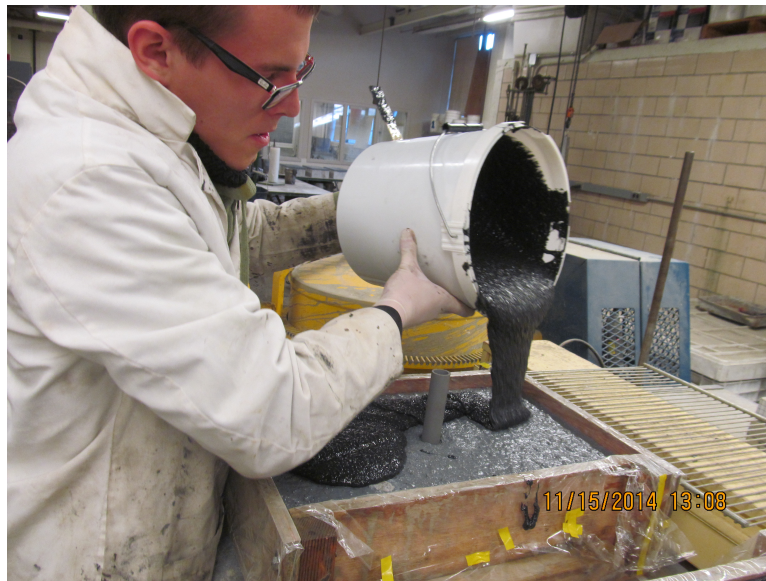
Figure 4-1. Liquid elastomer is poured onto a primed lightweight concrete block that will be used for compression testing.
