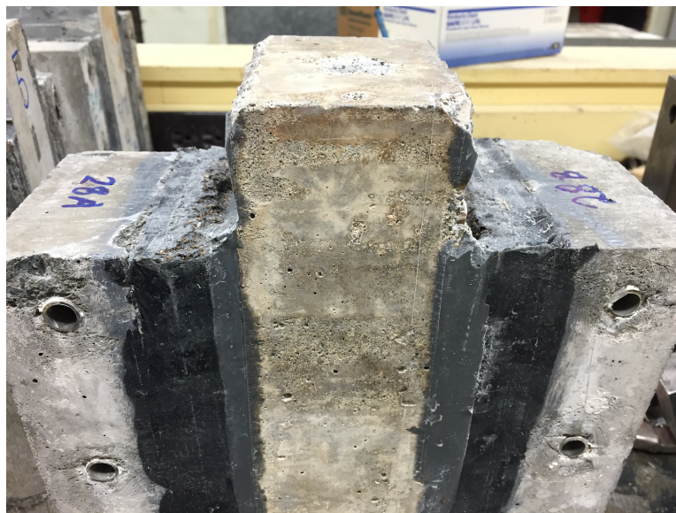
Figure 4-6. A Complete Shear Specimen.
