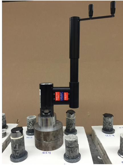
Figure 5-1. Tension Pull-off Test Apparatus.
