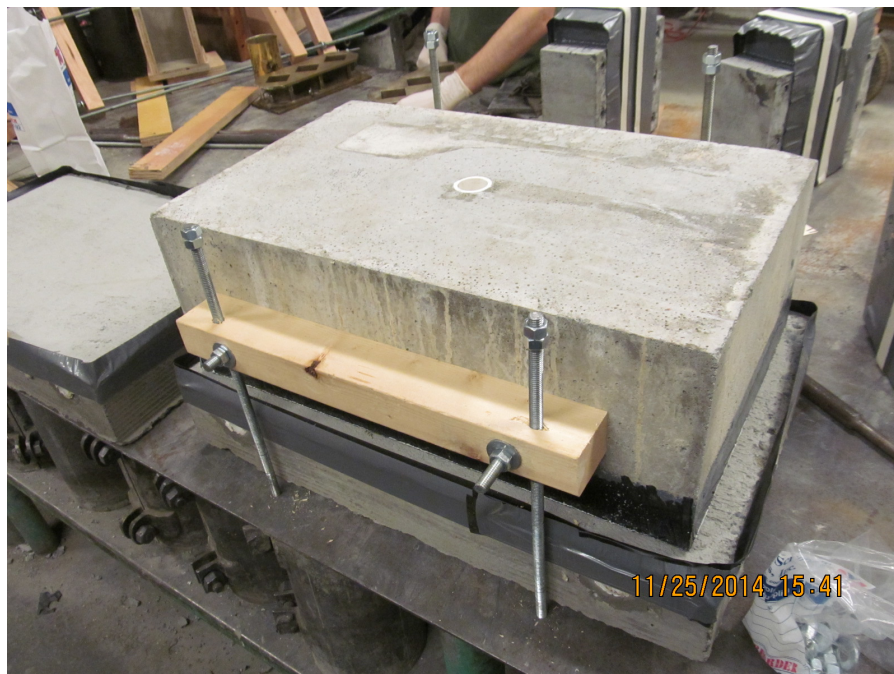
Figure 4-2. A plinth inverted over a concrete slab awaiting DexG application. A wood-reinforced duct tape barrier creates a dam for the DexG to flow into. The wooden reinforcing is not shown.
