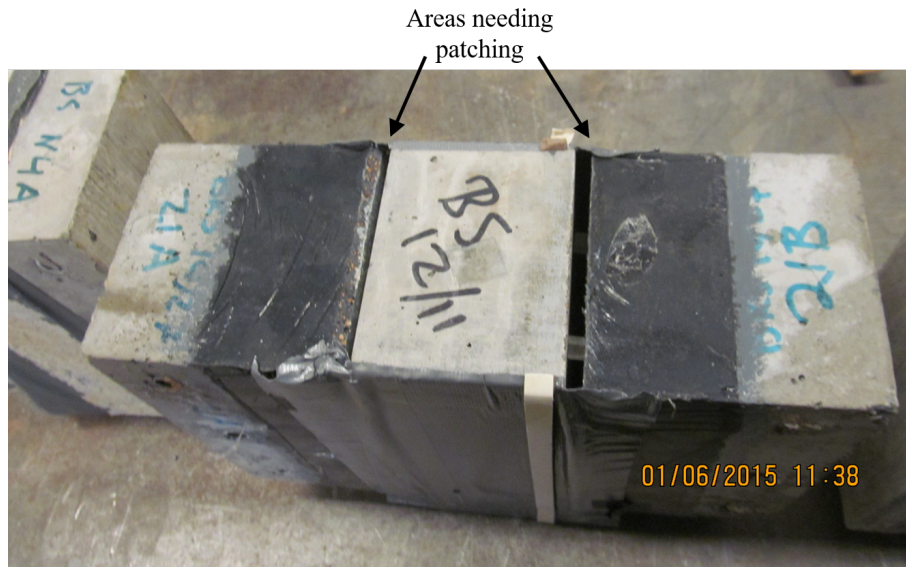
Figure 4-5. This double shear specimen required patching when the DexG did not flow all the way through the quarter-inch gap.
