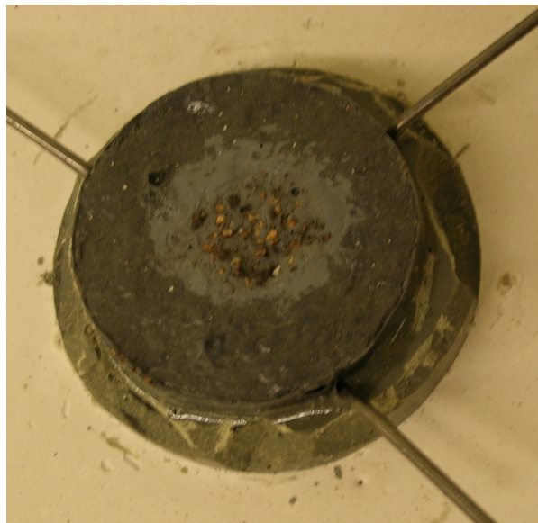
Figure 6-3. Tension Failure Surface Showing Failure in Corkelast at P.A.T. Test.
