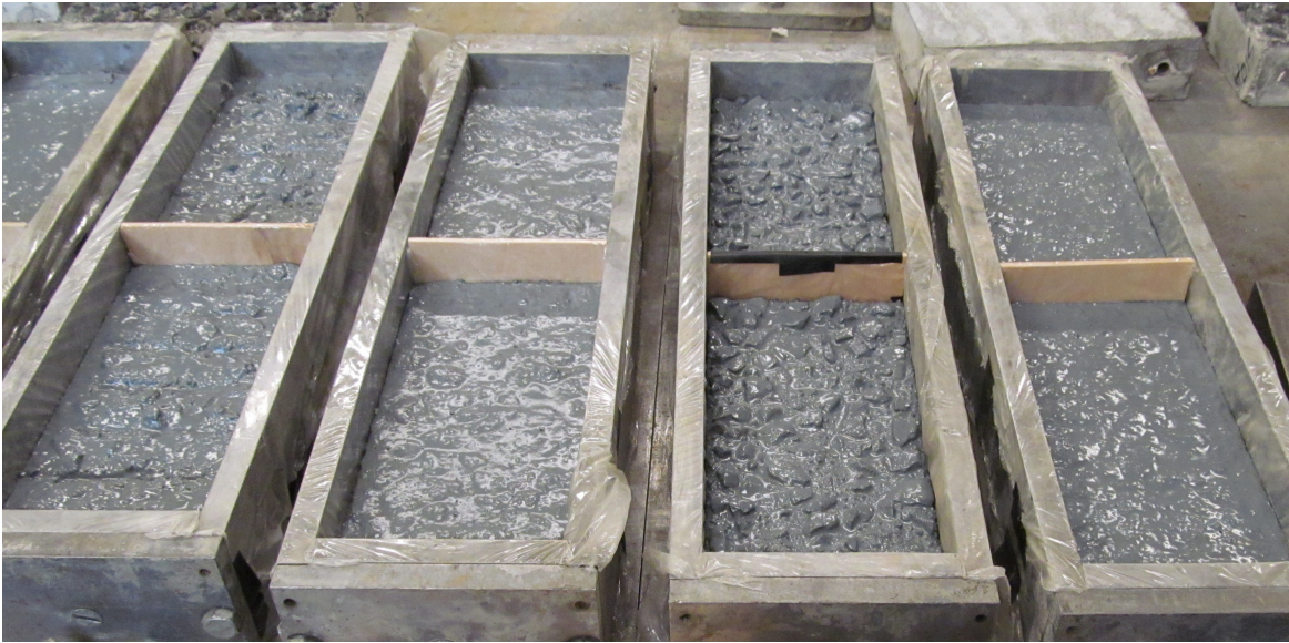
Figure 5-8. The four surface finishes tested were (from left to right) tined, sand-blasted, exposed aggregate and pressure-washed. They are shown primed, awaiting elastomer.
