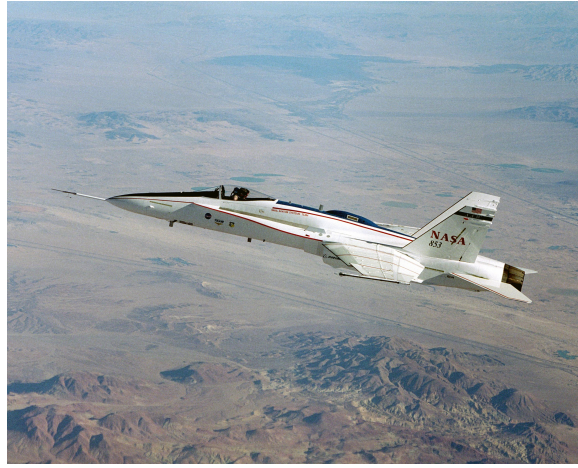
Figure 4.3: F/A-18 HARV TVCS aircraft in flight.
