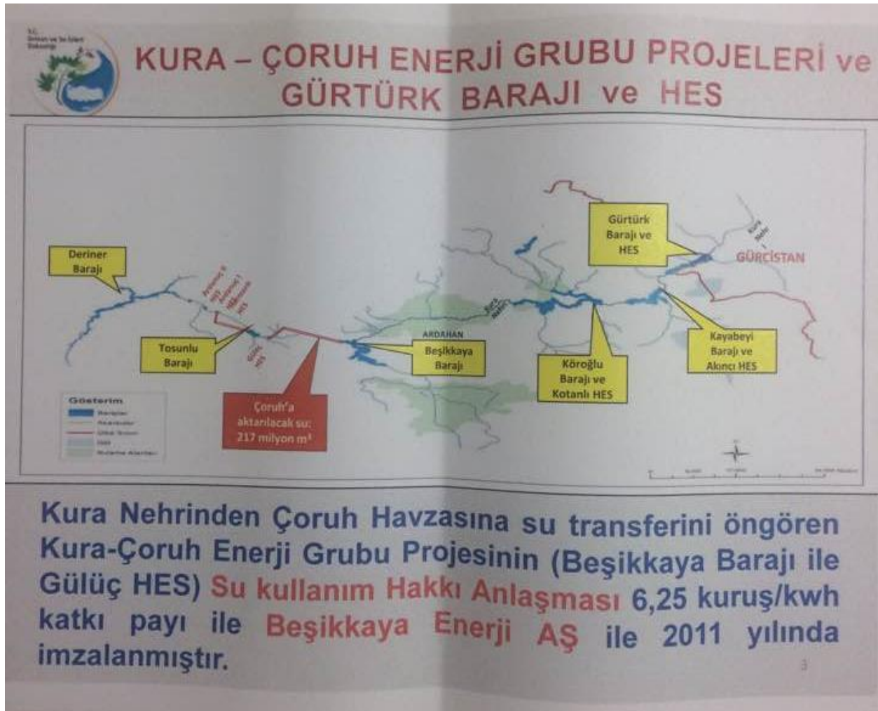
Figure 5.1 Map of existing and planned dam and hydropower projects in the Turkish portion of the Kura River Basin, including water transfer to the Çoruh River (in red) (Photo credit: Sanal Basın, 2018)
