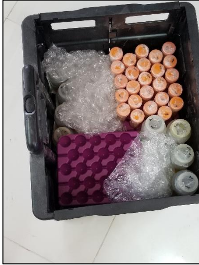
Figure 4: Modified shaker constructed from a foldable grocery cart on wheels, rolled by hand for entire shaking period.
