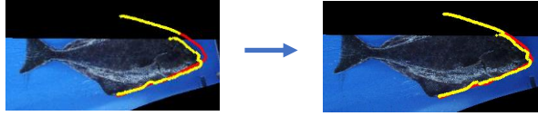
Figure 4.6: Contour refinement. An affine transform is estimated to minimize the distance between generated contour segments (red) and projected contour segments (yellow) for each two adjacent contour segments.
