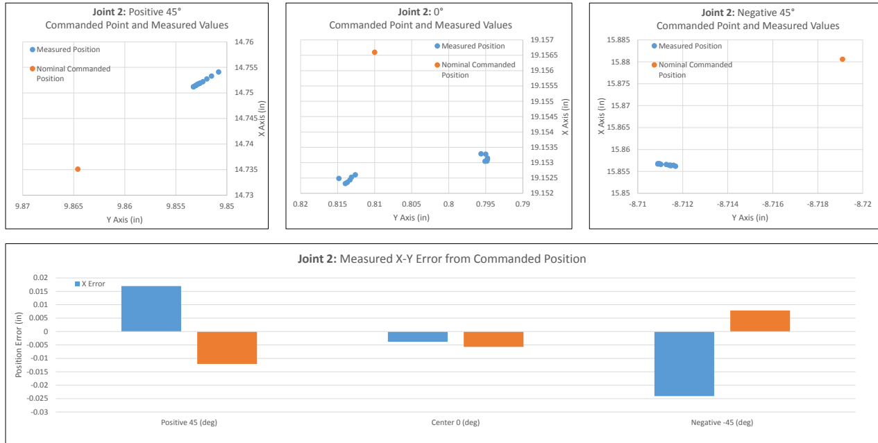
Figure 3.8: Top Left: Measured and nominal command to +45 degrees. Top Middle: Measured and nominal command to 0 degrees. Top Right: Measured and nominal command to -45 degrees. Bottom: Measured X-Y error from commanded position.
