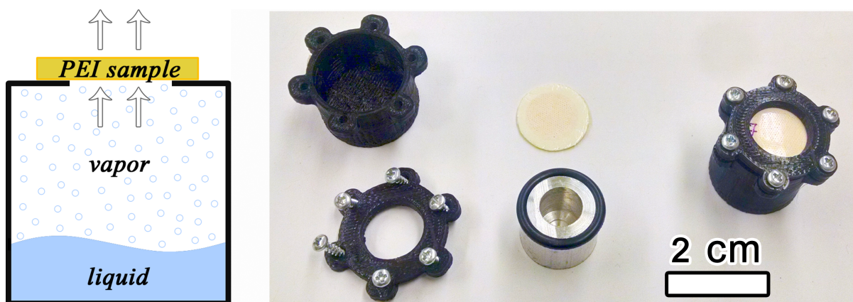
Figure 2.10: Vapor diffusivity test apparatus diagram and photograph of disassembled/assembled canister system.
