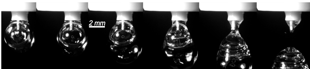
Figure 9.16: An air bubble inside a water droplet. Notice the difference in shape and wall thickness as compared to the soap bubble. The droplet has more mass when it detaches from the nozzle due to the higher surface tension of pure water.
