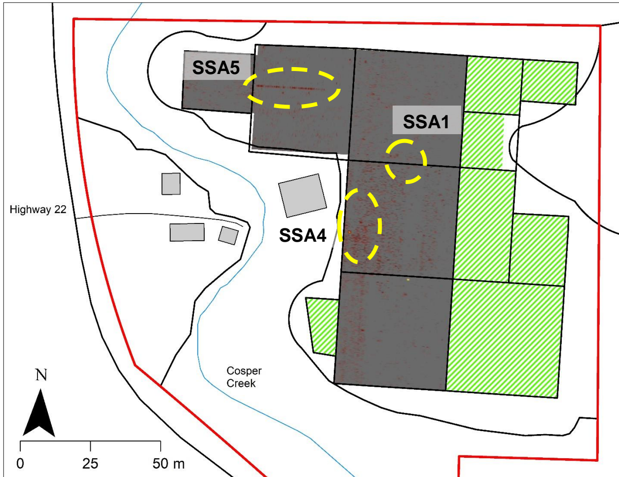
Figure 6.26 Amplitude map of July 2016 GPR results at 55 cm below surface.
