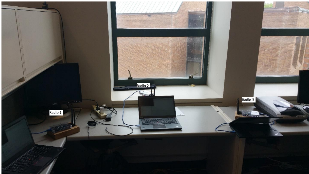
Figure 24: Picture of experiment set up. Radio 1 and 3 are clients, Radio 2 is AP.
