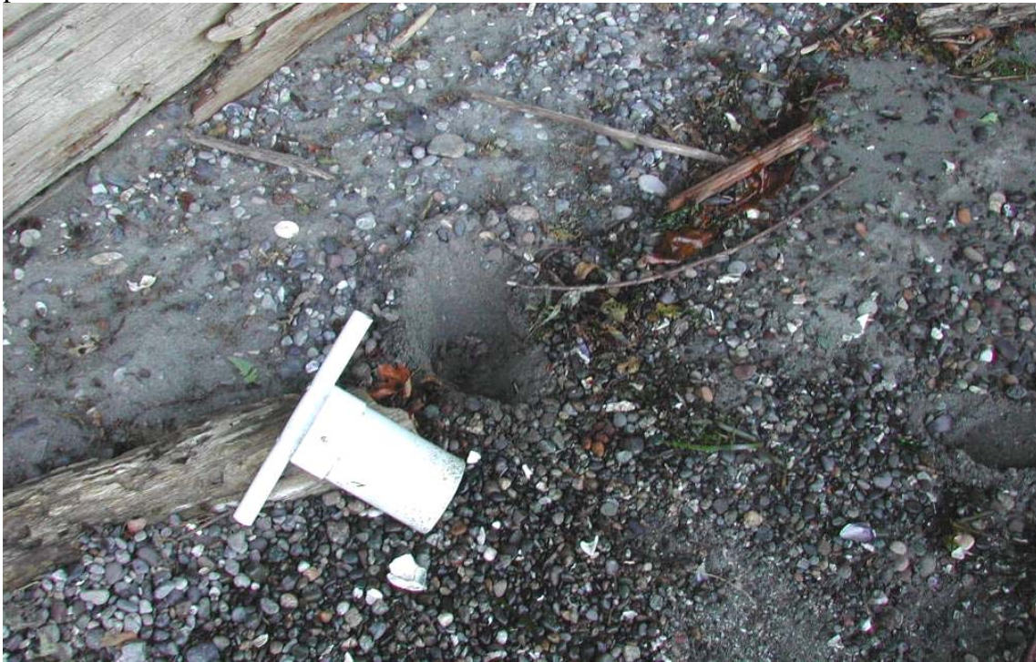
Figure 6. 10 cm diameter core used for sampling benthic invertebrates to a 15 cm depth.
