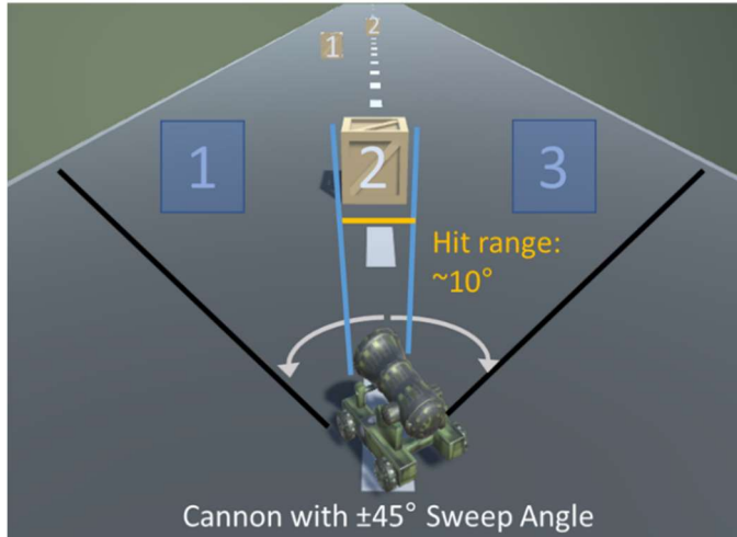
Figure 4.2 Visualization of the Cannon Task in Unity. Band power in Beta (10-30Hz) was used to rotate the cannon in place with 90-degrees of swing. Two thresholds, low and high, defined the beta power values that yielded no, counterclockwise, or clockwise rotation of the cannon. Power estimates completed by the TDT were updated each frame of the Unity task. Projectiles were launched when a countdown timer reached zero. If the projectile collides with the target box, then the API triggers the TDT to deliver stimulation across specified electrodes.
