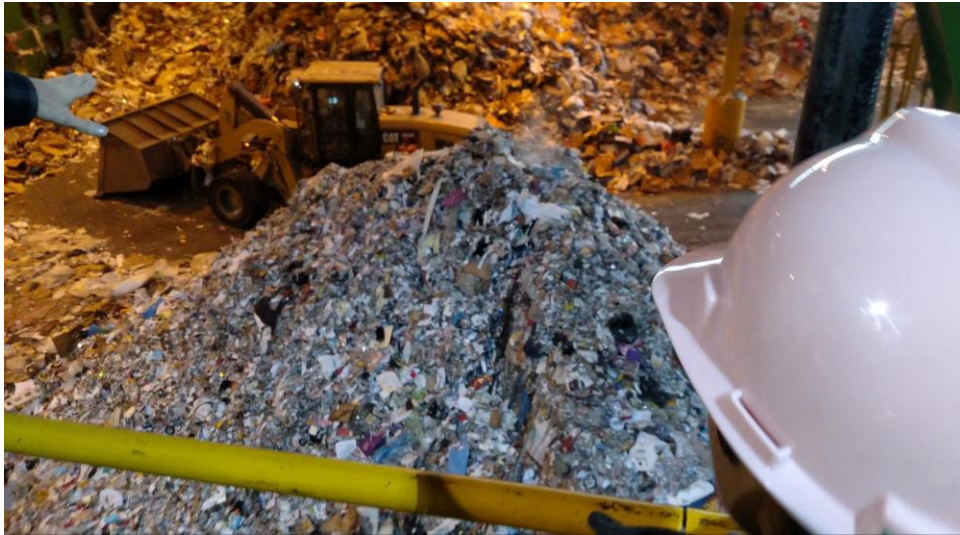
Figure 1-2. 3/8 minus material ready for baling.
