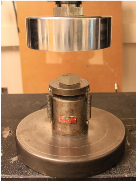
Figure 4-7. INSTRON 5585H outfitted with spherically seated bottom bearing plate.
