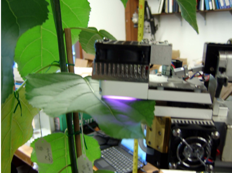
Figure 3.6 Setup measuring CO 2 uptake with a Li-Cor LI-6400. A portion of the intact leaf is illuminated and flatly clamped within the cuvette in the middle of the photo.
