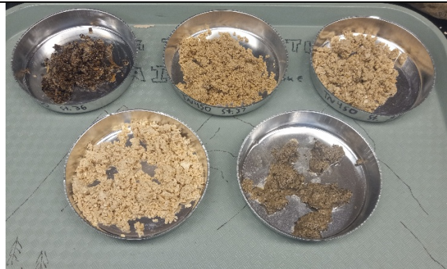
Figure 6. Sediment samples inside the lab after drying. Sediment on the top left is from station 36, top middle is station 37, top right is station 38, bottom left is station 39, and bottom right is station 35. Composition of each sample is described below in results section.
