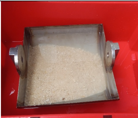
Figure 5. Sediment inside the sediment grab claw immediately after being brought up from the seafloor at Station 39.
