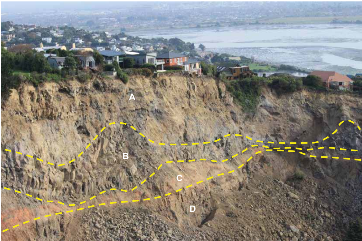
Figure 4.4: From Canterbury Earthquakes 2010/11 Port Hills Slope Stability: Risk assessment for Redcliffs [69]: Geologic units at the Redcliffs cliff face: A) Basalt lava breccia, B) Columnar jointed basalt lava and breccia, C) Epiclastics, and D) a second layer of basalt lava breccia.
