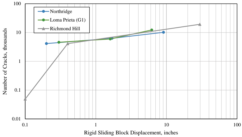
Figure 5.111: Number of cracks in the BPM simulations with rigid sliding block displacement for the Northridge, Loma Prieta, and Richmond Hill ground motions.
