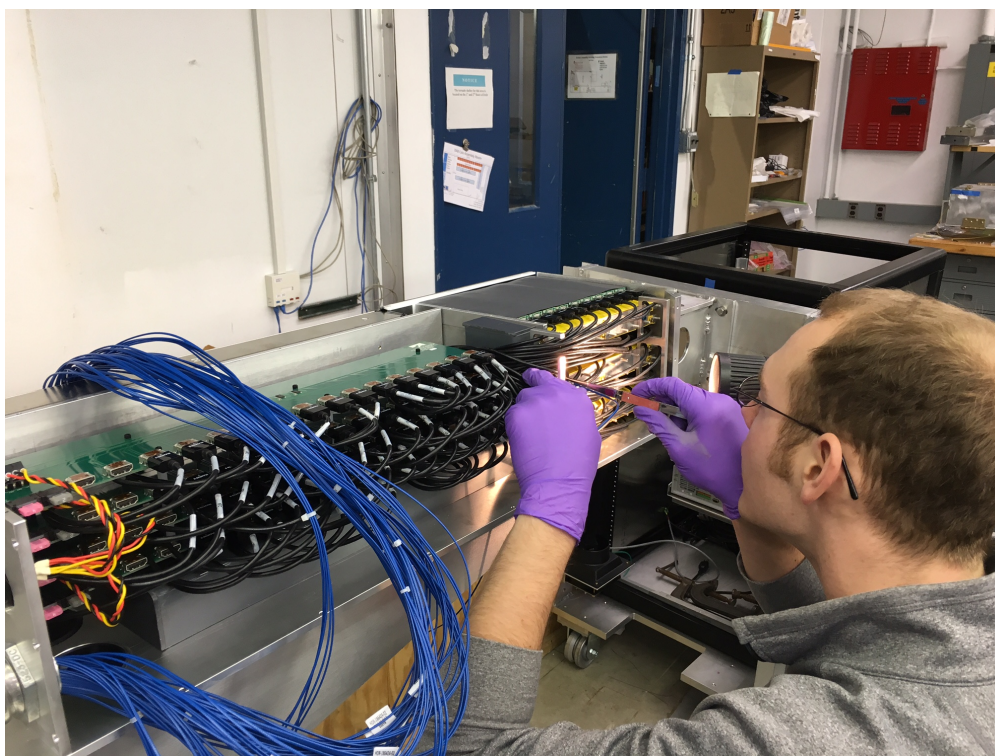
Figure 1: The author assembling one of the Muon g - 2 calorimeters. The active volume is at the right where a piece of black Tedlar rests on top of the array of \text{PbF}_2 crystals. The black HDMI cables provide communication and bias voltage to the SiPMs. The blue signal cables to the left have yet to be plugged into the SiPMs.
