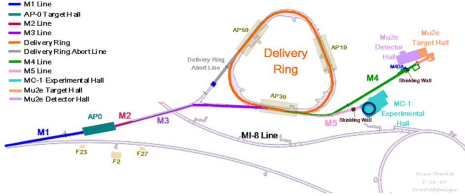
Figure 2.1: Schematic of the Fermilab beamline leading to the Muon g - 2 storage ring. Bunches of protons at 8 GeV from the M1 line in the lower left are smashed into a target in the AP-0 Target Hall. Positive particles (pions, protons, positrons) at 3.1 GeV/c are selected; the pions decay in flight into polarized positive muons. After four turns in the delivery ring, the time-of-flight difference between the muons and protons is large enough to extract the muons down the M5 line to the g - 2 storage ring and kick the protons into a beam dump. Image reproduced from [50].
