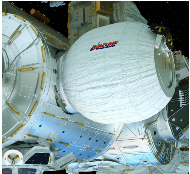
Figure 12: A rendering of pneumatic structure, by Bigelow Airspace, attached to the International Space Station. (Bigelow Airspace/NASA, space.com)
