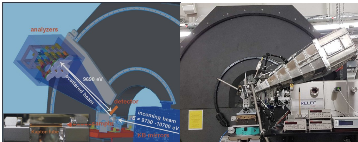
Figure 8. (Left) Design rendering of the P01 IXS/XRS 12-element spectrometer in a forward scattering geometry 26 (Right) Photograph of the P01 spectrometer in a back scattering geometry. A rigid enclosure provides a He flightpath through the spectrometer 21 .
