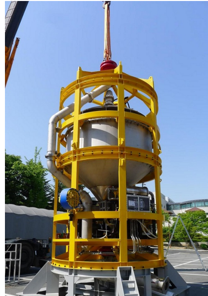
Figure 3.10. Korean collector “MineRo” and pump system. The figures are cited from Lee et al. (2014) and Service (KOCIS) (n.d.).
