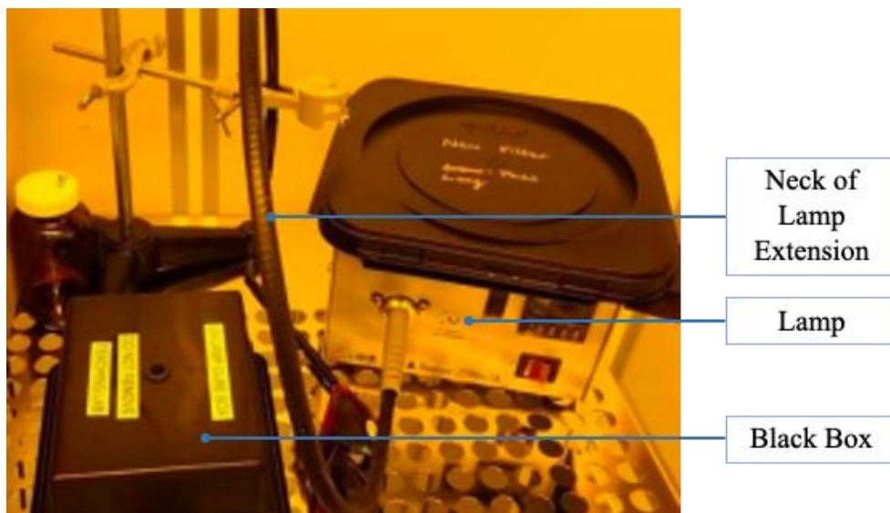
Figure 6. Set up of high-intensity UV BlueWave 200 lamp at WNF.
