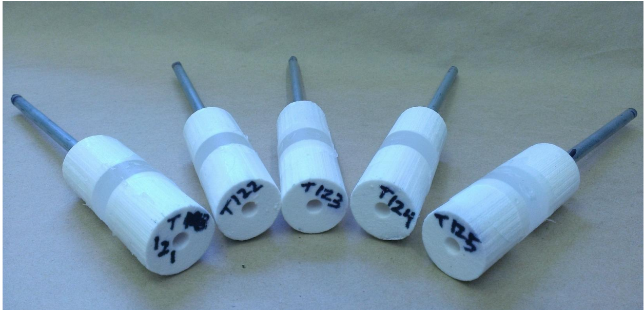
Figure 5: Assembled models. The 6 shown are 180 degree models with various intervertebral joint lengths. The moment arms have been attached with cyanoacrylate.
