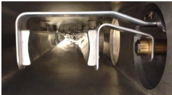
(a) Kicker plates positioned radially inward and outward of the muon storage region provide a pulsed vertical magnetic field to shift the beam onto its nominal orbit.
