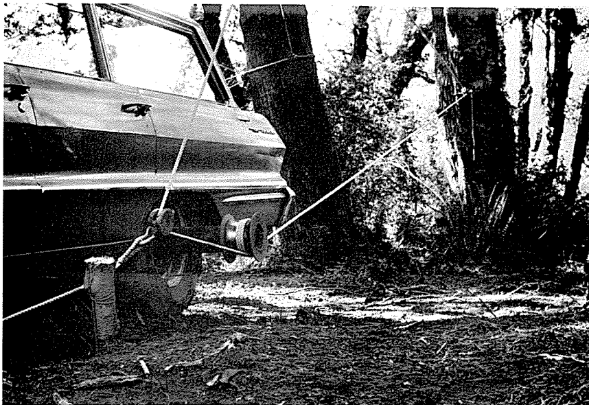
Fig. 4. Gypsyhead which provided power for lowering and lifting the sampling net.
