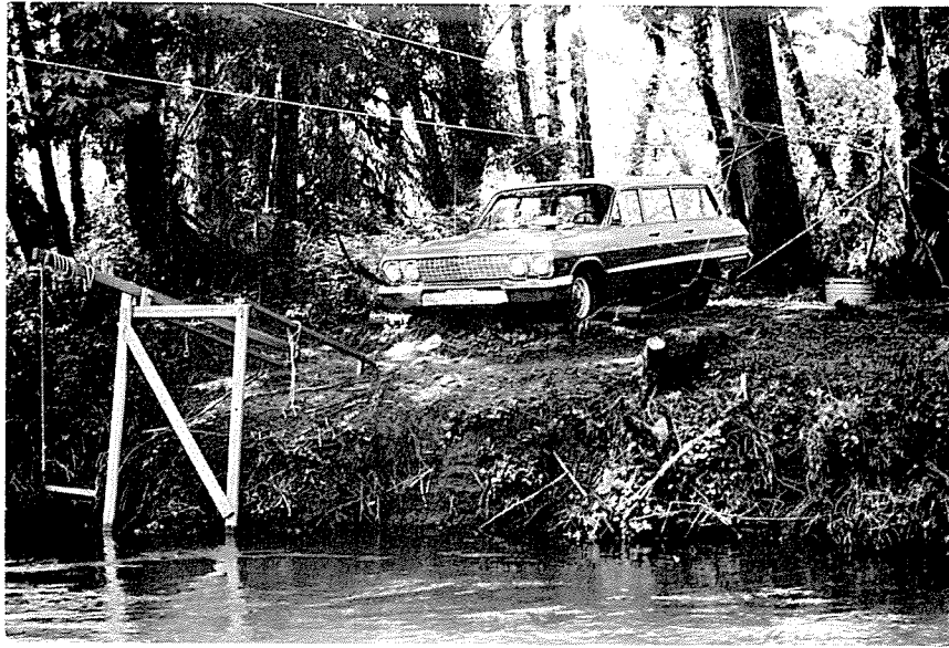
Fig. 3. Second-hand automobile adapted as a power source for shore-based net sampling of the Lower Quinault River. Lever for lifting live tank appears at left.
