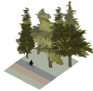
The creation of a two-way bike lane with minimal space on either side creates a wide enough corridor for first responder vehicles in an emergency.
