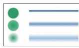
Figure 2. Fuzziness as applied to points (left) and lines (right), from MacEachren et al 2012)
