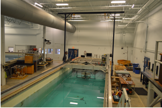
Figure 4.3: Image of the towing tank at the Chase Ocean Engineering Laboratory at UNH
