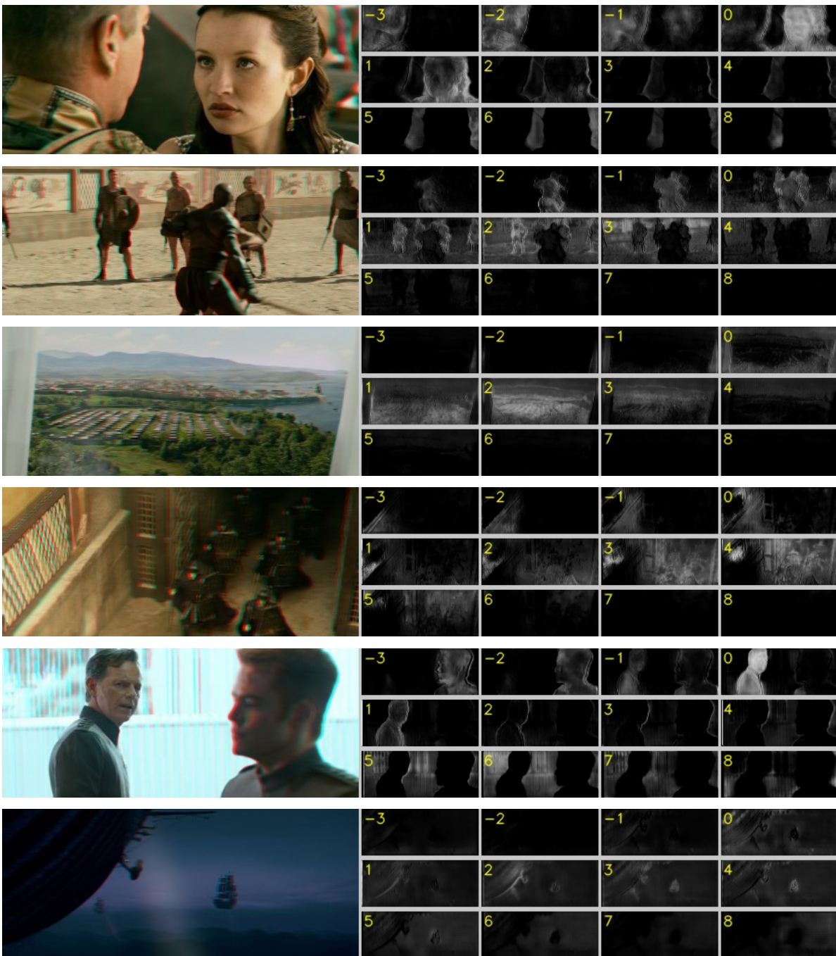
Figure 4.4: Qualitative results. Column one shows an anaglyph of the predicted 3D image (best viewed in color with red-blue 3D glasses). Each anaglyph is followed by 12 heat maps of disparity channels -3 to 8 (closer to far). In the first row, the man is closer and appears in the first 3 channels while the woman is further away and appears in 4th-5th channels; the background appears in the last 4 channels.
